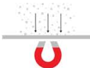
Short-range electromagnetic forces (Van der Waals) enable Dycem to attract, collect and retain over 99% of particles.
